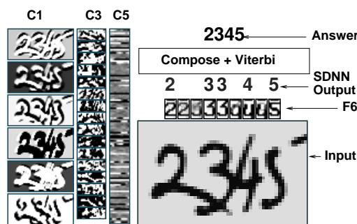
Fig. 25. An example of multiple character recognition with SDNN. With SDNN, no explicit segmentation is performed.
